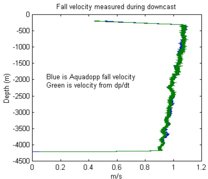
Figure 7 – Vertical velocity measured by the Aquadopp and calculated from the differentiated pressure data during the downcast
