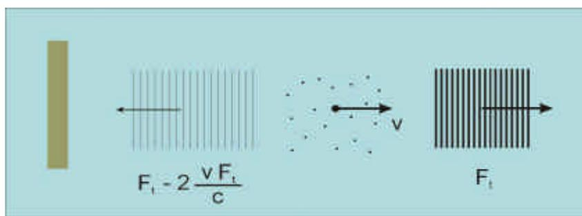
Fig. 1 – Acoustic backscattering
