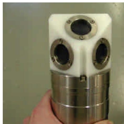
Fig. 3— The 6000-m Aquadopp transducer head. The three "eyes" are the acoustic transducers. The white portion is the transducer housing, which is made from a plastic material. All metal parts are made from Titanium gr. 2
