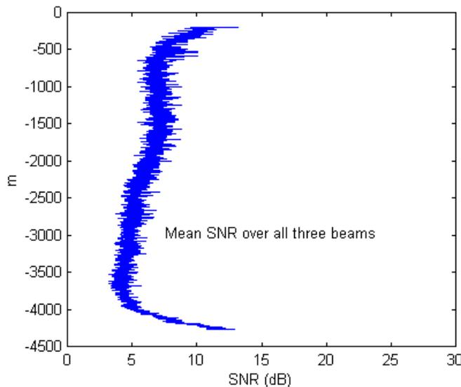
Fig. 6 – SNR data collected from the surface to the bottom in 4500 m of water in the Sargasso Sea. Data collected during transect from Woods Hole to Bermuda.
