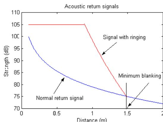
Fig. 2 – When the return signal is weak, the acoustic ringing dominates the measured signal for some time after transmit. To avoid getting bad data, the ringing must be allowed to die out before sampling can start. Since the echo from the water gets weaker with time, the net effect of ringing is to reduce the sensitivity of the Doppler current meter. Ringing is specific instruments where the underwater housing is made from metal
