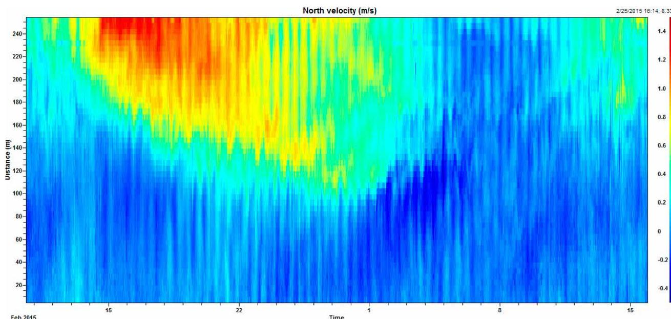
Color contour plot showing current data (as a function of depth and time) from a deployment off the coast of Trinidad. A ring current spinning off the North Brazil Current (and impacting the project area) was clearly visible in the data.
