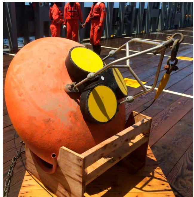
*Coastal Dynamics Limited chose Nortek's Signature55 to collect high resolution current data in the water column off the coast of Trinidad.*
