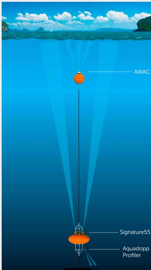
*Signature55 mounted on an elliptical buoy. This buoy has an optional pocket where users can integrate the Aquadopp Profiler for higher resolution current profiling. The AWAC is mounted on top of the spherical buoy.*
